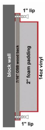
Screw directly through 1" nailer lip into your wall every 8-10" for best results. Make sure you use the correct type of screw for your wall material. This process is often more difficult as screwing into your block wall every 8-10" is more difficult than the next option noted below.
