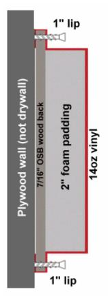
Screw directly through 1" nailer lip into your wall every 8-10" for best results. Make sure you use the correct type of screw for your wall material.
